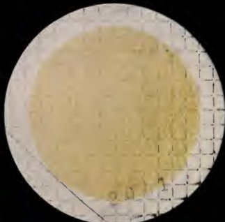
FILTER GETS THIS MUCH DEBRIS FROM TWO QUARTS OF NORMAL DRINKING WATER
