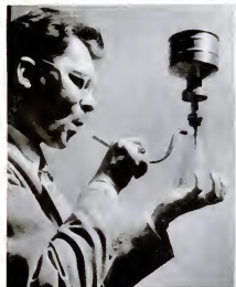
TRAPPING BACTERIA with newly developed filter (inside metal funnel), a bacteriologist sucks on tube to create a partial vacuum which pulls sample of water through filter and into conical flask below.
