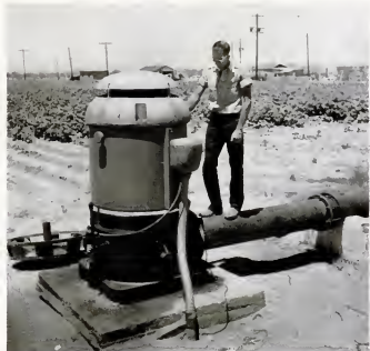
NONSTOP PUMPS , like this one on 600-foot well irrigating a cotton field, have left the much shallower well of Palos Verde Vista homes ( background ) bone dry.
