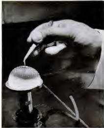
REMOVING FILTER from the funnel, tweezers are clamped on edge so bacteria trapped in middle will be undisturbed. Next, the filter is laid on pad filled with nutrient media, then wrapped up in Pliofilm.
