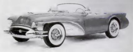
many Buick models. Right: the 100-inch wheelbase, 35½-inch-high experimental Wildcat II which will be shown around the U.S. this year for public reaction.
