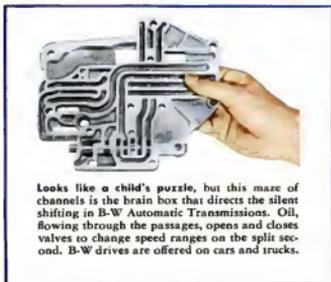
Looks like a child's puzzle, but this maze of channels is the brain box that directs the silent shifting in B-W Automatic Transmissions. Oil, flowing through the passages, opens and closes valves to change speed ranges on the split second. B-W drives are offered on cars and trucks.
