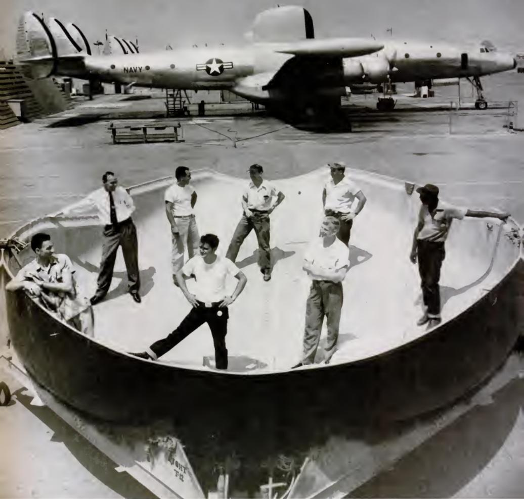
**BIGGER RADOMES FOR MORE PROTECTION.** The radar Super Constellation picket plane is an extremely vital unit for U.S. protection. It can warn the nation hours earlier of enemy air attack, because it has long range, high speed, plus more than six tons of electronic intelligence packed in radomes as big as swimming pools (like the bottom one pictured above).
