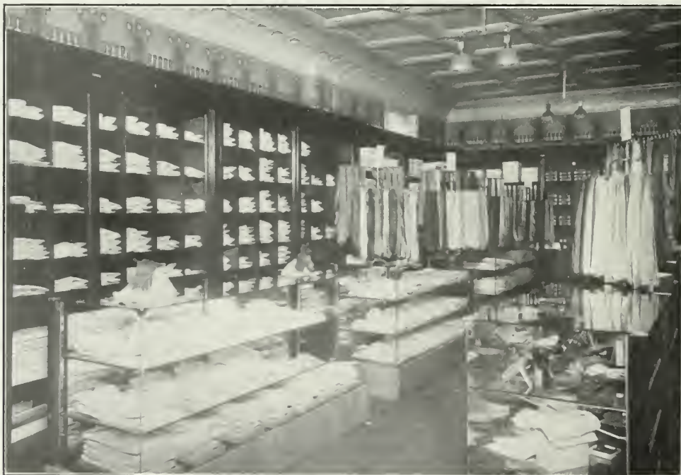
Interior view, furnishings section, Danfield-Bellinger store, 426 Yonge St. Arranged purposely to show shirt cabinet on left. This is 15½ feet long and 8 feet high and is divided into apartments, each about one foot square and in sufficient number to contain the range of regular sizes. It has glass sliding doors and has proved its value as a good stock keeper and display fixture. Cost, about $160 in mahogany-finished birch.
