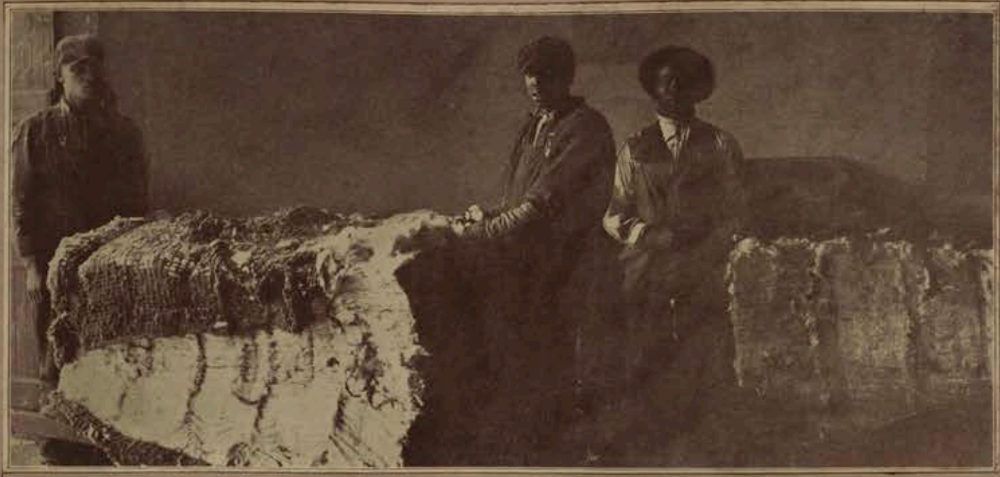
Cotton bales are inspected on their arrival at the mill and then thrown into a bale-breaker which tears the lumps and flakes apart.
