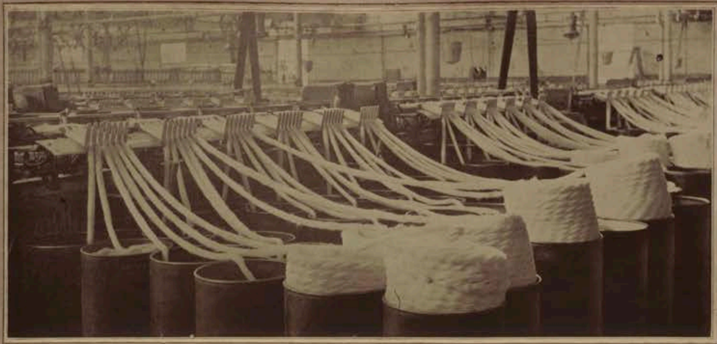
Six slivers are fed at one time into the "Drawing Machine" which combines them and draws them out into one sliver six times the original length. (Marshall Field & Company's Mill at Fieldale, Virginia)
