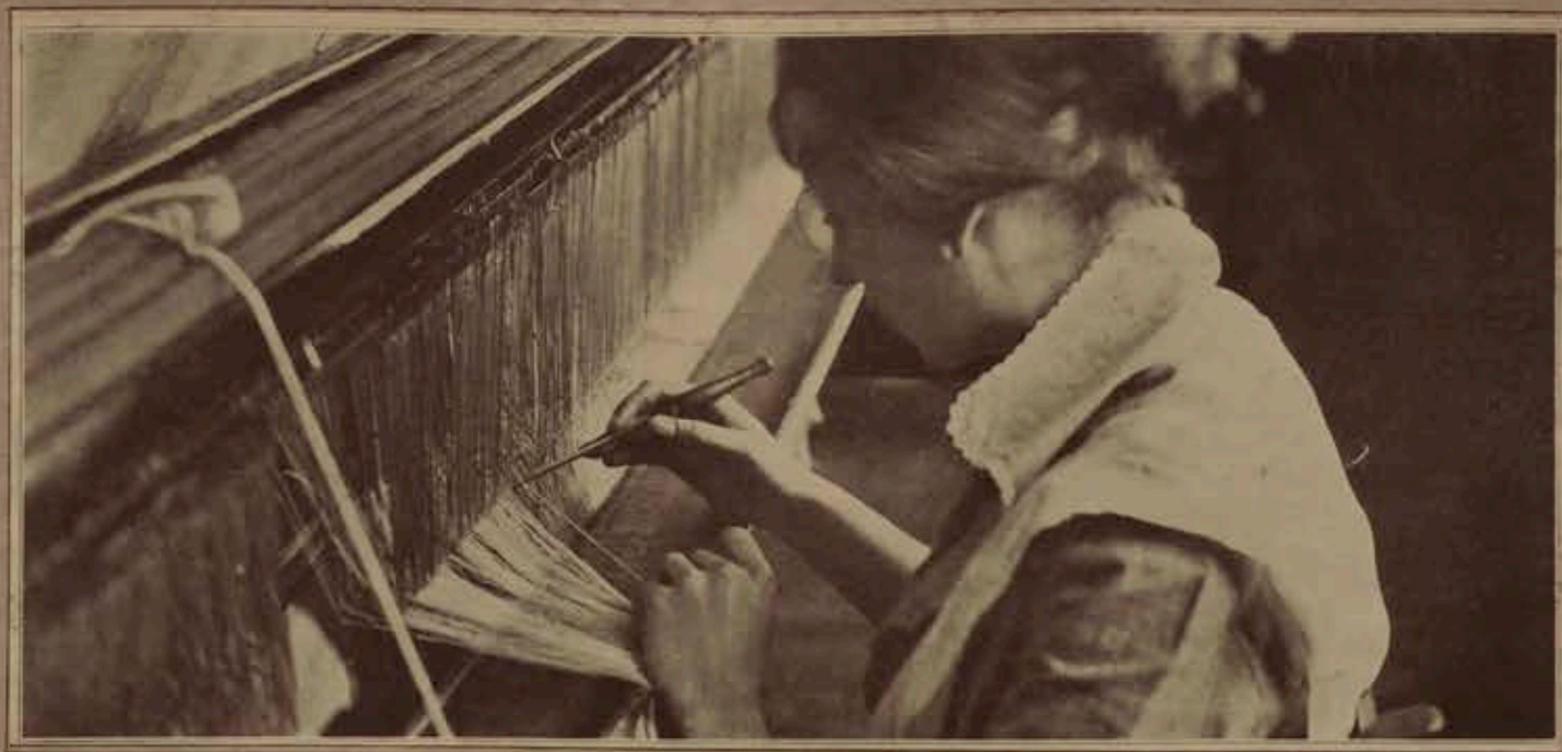
Drawing the warp threads through the eyes in the harness, of the loom, to enable them to be lifted or depressed as desired. In the Jacquard loom, each warp-thread is separately controlled.
